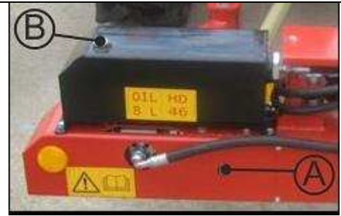
Picture 10 hydraulic system oil tank
