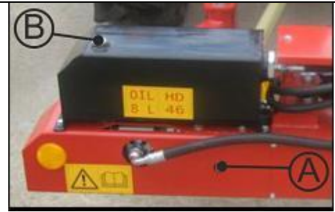
Picture 10 hydraulic system oil tank
